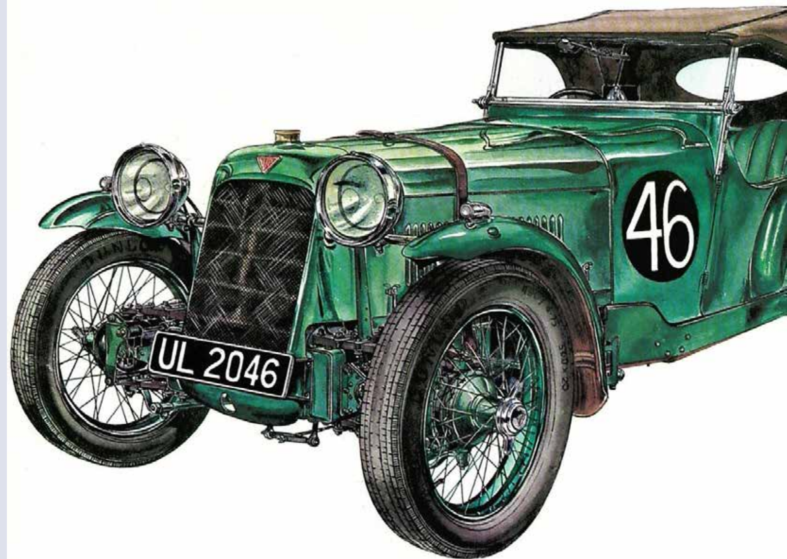
1929 Alvis Four cylinders, 68mm by 102mm, 1482cc; 75bhp supercharged, 50bhp unsupercharged; four forward gears and reverse; front wheel drive
