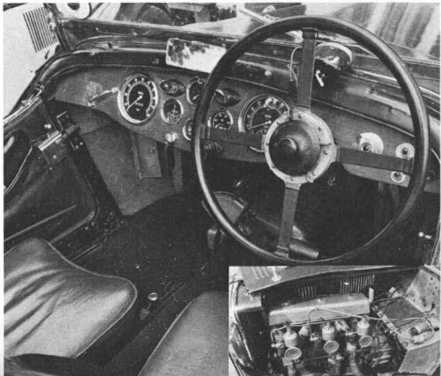
Above, an earlier run in Rivers Fletcher's Birkin replica Speed 25 showed Alvis integrity without coachbuilt weight. Below, interior of John Champion's SA Speed 20 with non-standard pre-selector box; inset, 2.5-litre 4-bearing six gave 83bhp on triple SUs.
