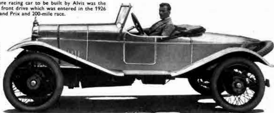
SUCCESSFUL BASIS—The fortunes of the company were founded on the 12/50 model, the racing version of which won the 200-mile race of 1923 at an average speed of 93.29 m.p.h. and nearly 24 m.p.g.
