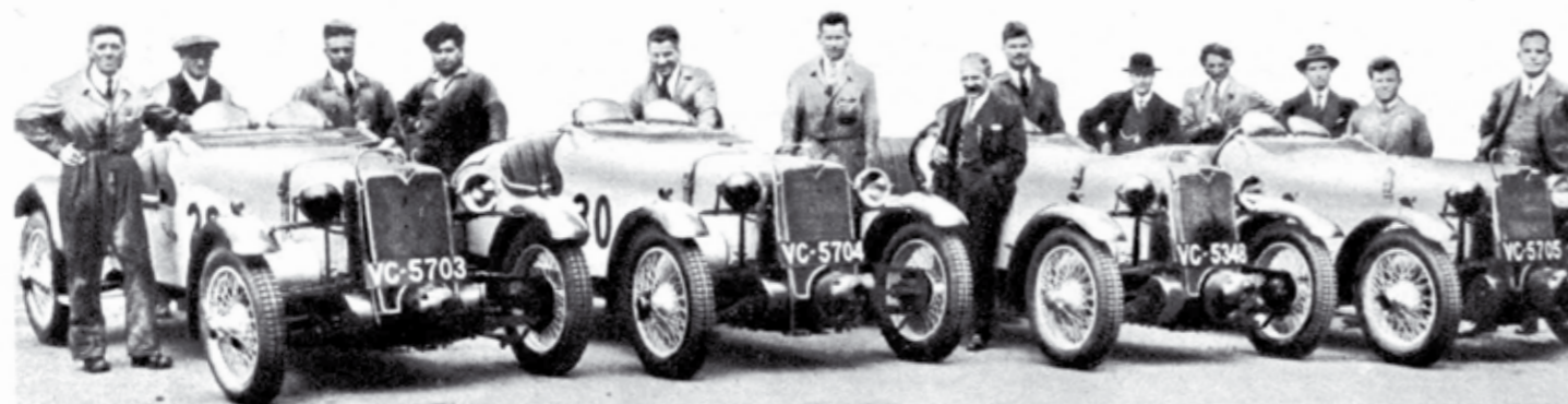
ADVANCED DESIGN —A team of 1928 sports car Alvis was entered for the T.T. race and advanced features of the design included independent suspension to all four wheels, overhead camshaft and supercharged engines.
