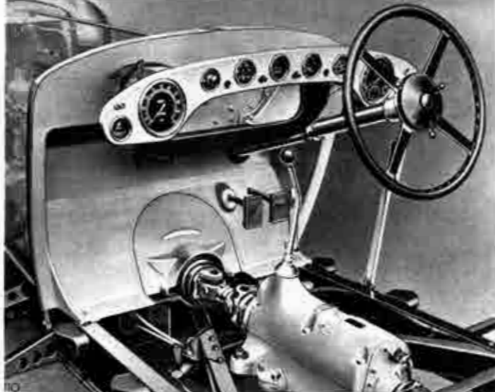
SPLIT BOX—In 1933 Alvis pioneered a four-speed all-synchromesh gearbox which, as shown in this illustration, was split on the horizontal centre line which made it possible to incorporate a centre bearing.
